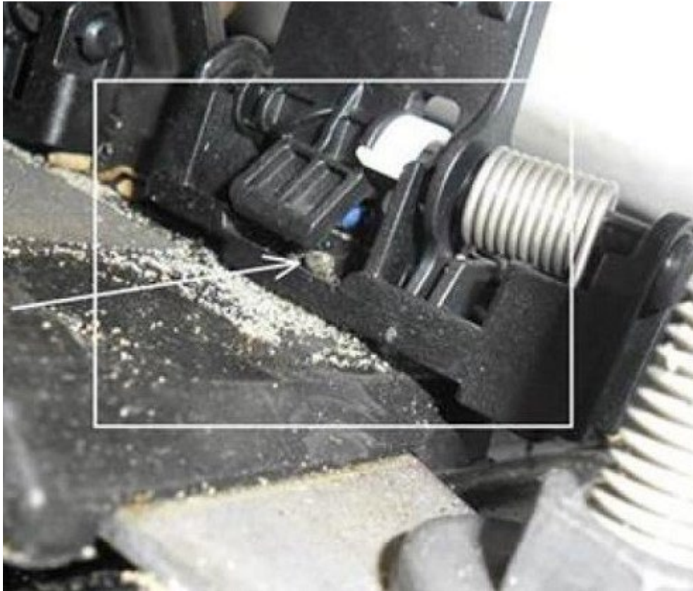
Figure 1: Dirt and debris interfering with the operation of the rear lid sensor.
