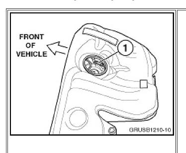
2. If no fuel pressure is present then remove the right side fuel tank access cover to inspect the fuel hose (1) for disconnection or damage. Refer to Repair Instruction REP 16 14 010 Removing and installing the fuel pump.
