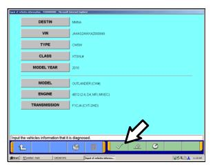
Confirm that all data matches the vehicle and click the check mark at the bottom of the page.
