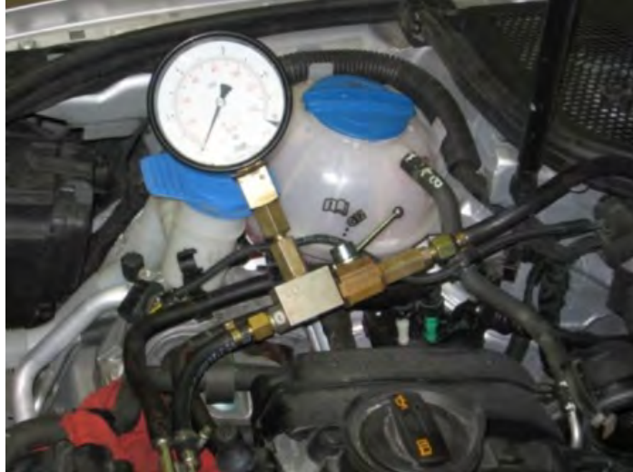
Figure 1. VAG 1318 gauge installed on an A3 2.0L TFSI.
