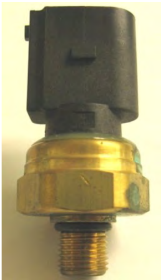
Figure 2. Improved fuel pressure sensor 06E 906 051 K.
