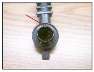
**Figure 1.** Incorrectly assembled drain hose, with locating tab pointing up.
