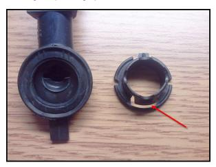
Figure 2. Hole in snap ring.
