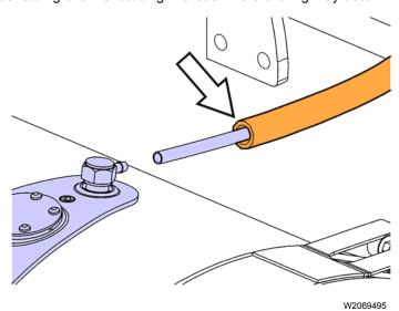
15 Route new vent-line from the fuel tank, under the deck plate, and to the filter (Left Side). 16 Install line on filter manifold (Left Side).
