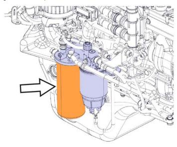
19 Attach fuel tank ventilation filter labels (21807860) as shown in the figures below.
