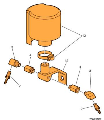
3 Install manifold and filter on exhaust stack bracket and tighten fastener to 140  $\pm$  25 Nm (103  $\pm$  18 ft-lb).
