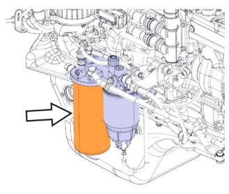
19 Attach fuel tank ventilation filter labels (21807860) as shown in the figures below.
