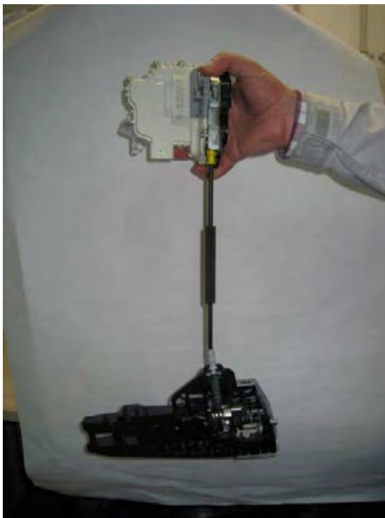
Figure 5. Do not turn the lock or the mounting bar.
