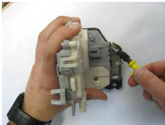
Figure 3. Holding the yellow sleeve in the lock.
