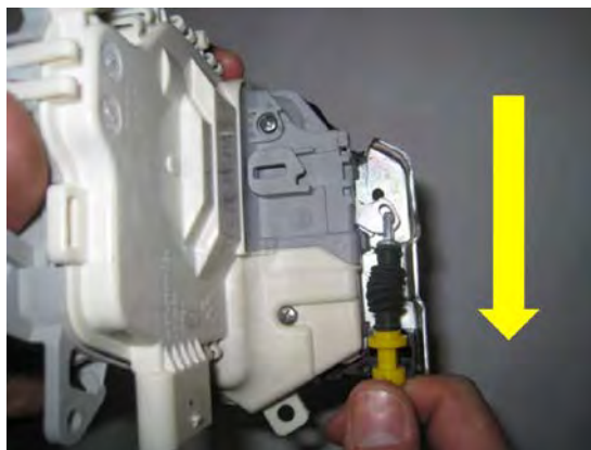
Figure 4. Pulling down the Bowden cable.
