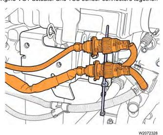
**Note:** Ensure the cable tie is in the end groove between connector flange and back shell as shown in figure below.
