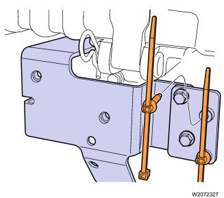
10 Connect and lock the engine VGT actuator and TSS sensor connectors together.
