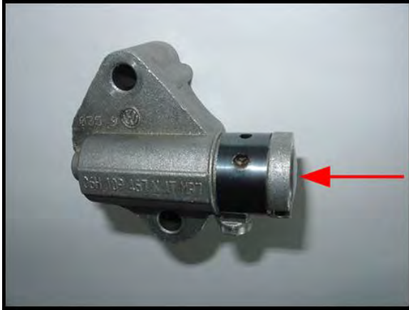
Figure 2) Timing chain tensioner incorrect
