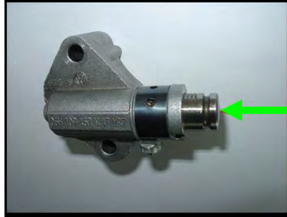
Figure 3) Timing chain tensioner correct
