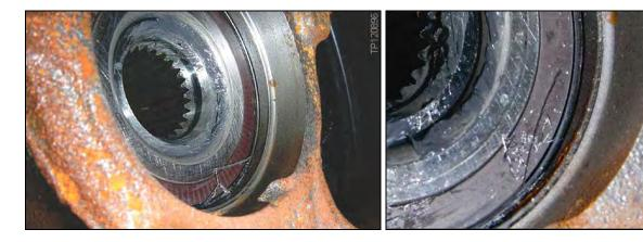
**NOTE:** Contamination on wheel speed sensor tone ring can cause intermittent errors.
