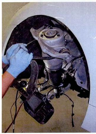
14. Unfasten and remove the 3 strut top mounting nuts (N).
