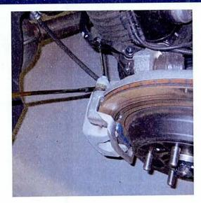
Pump the brake pedal 3 times and hold the pedal down, to pressurize the system.
