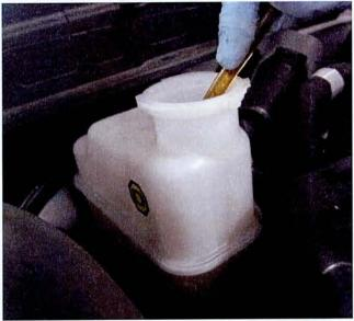
Fill the reservoir to the MAX line using DOT4 brake fluid.
