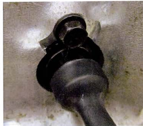
Early production sensor without retaining clip
