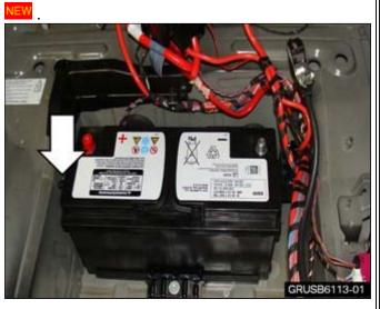
Before mounting the battery in place, make sure the battery vent hose is connected as indicated by the arrow. The short end of the elbow should be connected to the battery to gain some extra clearance.
