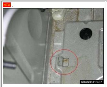
Important Note: Before mounting the battery in place, bend the metal tab down flush with the battery tray. In some cases, a longer battery vent tube must also be installed in order to facilitate the larger battery.
