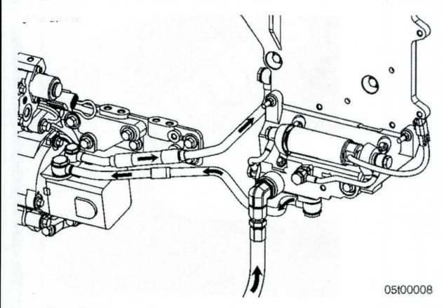
New Fuel Pump Gear Pump with Revised Fuel Line Locations
