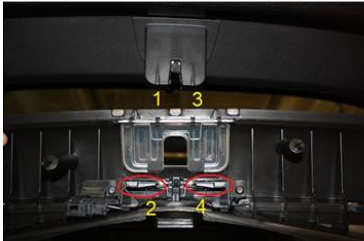
Figure 7. Inside vehicle view of rear lid latch showing location of G526 (2) and G525 (4) on rear sill trim, and contact points (1 and 3).
