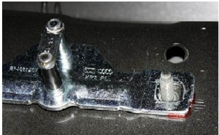
Figure 6. Manual lid style striker plate adjustability and serrated indicators.
