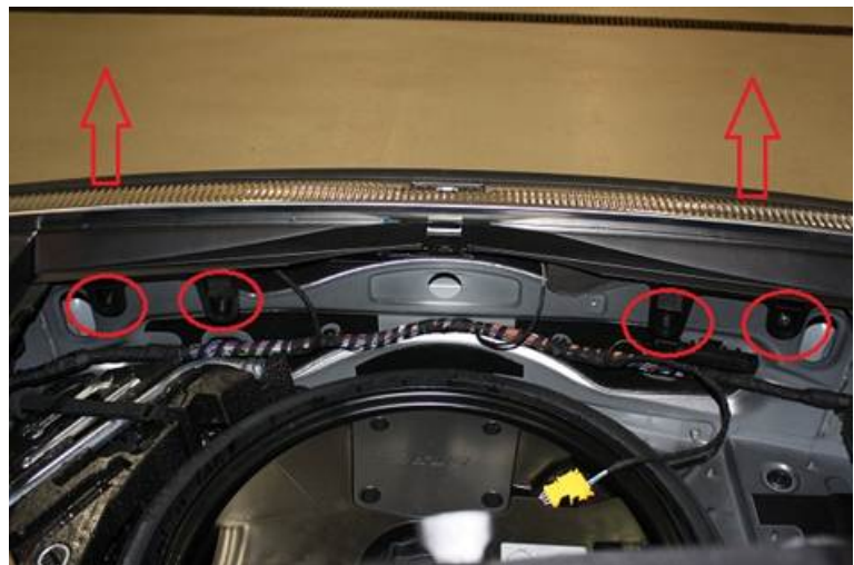
Figure 2. Rear cargo area trim plate removal in the Audi Q7. The T25 Torx® screws to be removed are circled in red.
