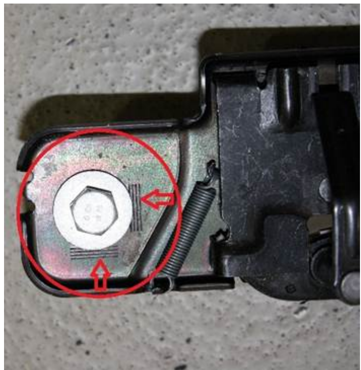
Figure 4. Power lid's motorized striker plate adjustability and serrated indicators.
