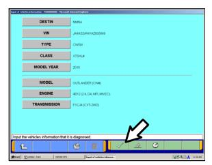
i. Confirm that all data matches the vehicle and click the check mark at the bottom of the page.
