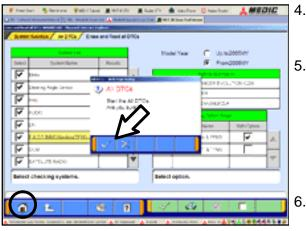
c. The "System List" list on the left side of the screen will have all selections checked. <u>Do not</u> change these selections. DTCs may be set if the vehicle is equipped with options that are unchecked.
