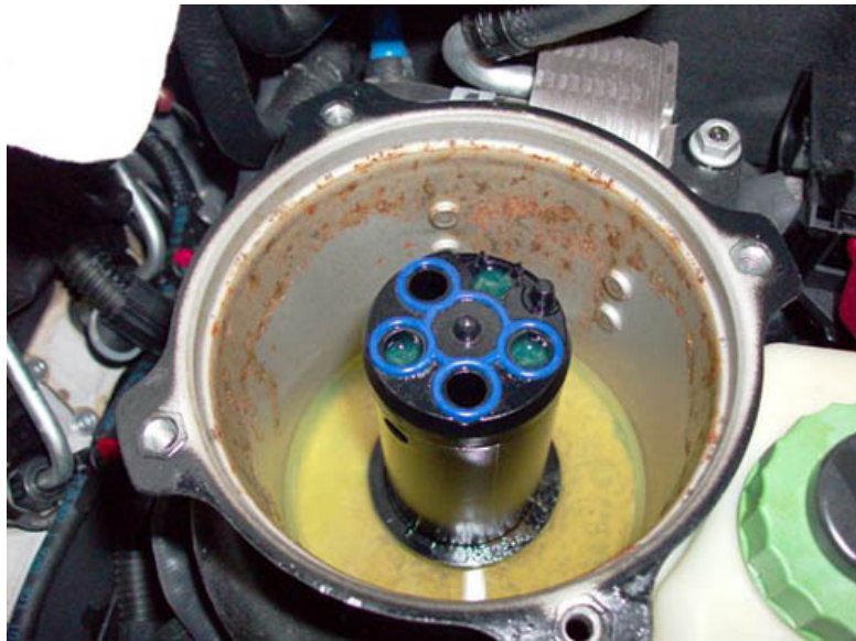
Figure 2. Example of rust in fuel system caused by water contamination.
