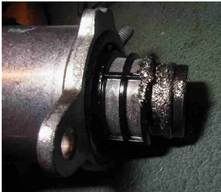
Figure 4. Metallic debris on screen of N290 metering valve.
