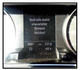
Figure 1. Audi Side Assist warning in DIS
