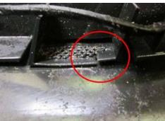
Figure 3. Mounting bracket broken
