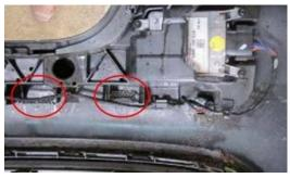
Figure 2. Mounting bracket for one of the ECUs.
