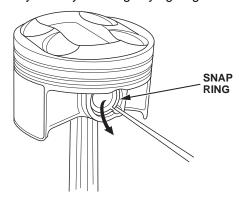
40. Put on gloves, heat the piston and the ends connecting rod to about 158°F (70°C), then remove the piston pin.
