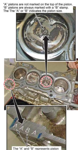
size. Piston sizes can be mixed in an engine block assembly.
