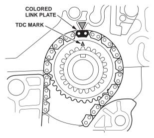
Set the oil pump chain on the oil pump chain sprocket with the punch mark aligned with the center of the colored link plates, then install the oil pump chain sprocket to the oil pump.
