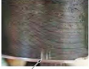
SCRAPES, DEEP SCRATCHES, OR DAMAGE
