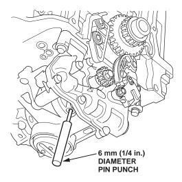
27. Loosen the oil pump sprocket mounting bolt.
