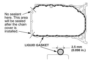
78. Install the oil pan to the engine block.
