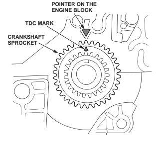
Install the oil pump chain on the crankshaft sprocket with the colored link plate aligned with the TDC mark on the crankshaft sprocket.
