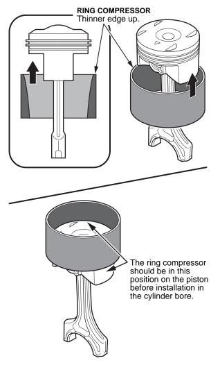
56. Set the ring compressor on the piston bore, then push the piston in with your hands.
