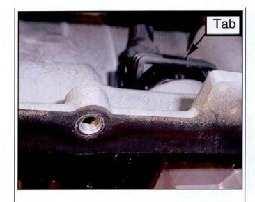
Use an 8mm or 5/16" hex socket and remove the drain plug and drain the ATF. Reinstall the drain plug.
