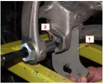
10. Using the drill, remove damaged threading by drilling into nut screw seat (2) until the drill bit comes out of the other side by a few millimeters (3).
