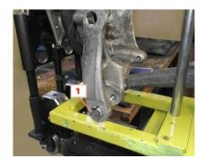
2. Using a clean cloth and a suitable degreaser, clean hub holder unthreaded seat (A).
