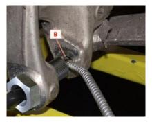
7. Using a suitable drill, install the drill bit supplied and insert it in through the **Heli-coil Insertion Centering Tool** No. **900000223** (1), until drill bit tip is fully contacting the bolt hole (B) as shown in the illustration below.
