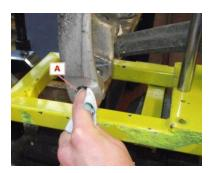
3. Insert special tool No.900000223 "Helicoil Insertion Centering Tool" (1), without stop nut, inside the unthreaded seat.
