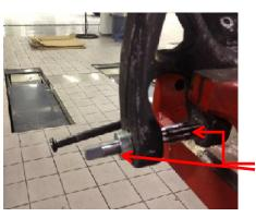
Side View of how the Tap will look passed through the bushing driver inserted into the non-threaded end of the knuckle assembly. Ensure Tap is level before beginning threading process
