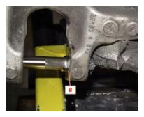
16. Thoroughly clean and remove any residual metal from the bolt hole (B).
