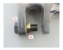
6. Using commercially available cutting oil, lubricate the seat of hub holder bolt hole (B).
