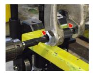
9. Place metal protection plate (1) between hub holder and lower lever, behind hub holder bolt exit hole (2)
