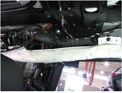
Figure 1. Sunroof frame and mounting bracket above left rear door.
