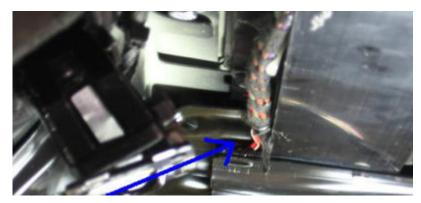
**Figure 4.** Wire, pinched between the sunroof frame and the bracket that holds the frame to the body on the left side of the vehicle above the C-pillar. Photo taken from the rear hatch opening.
