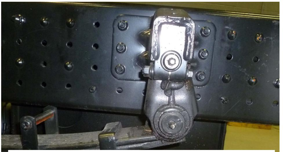
If additional clearance is needed to remove the tank, support the rear differential housing with a suitable jack. Remove the upper spring pins on both left and right sides. Lower the rear differential housing until the needed clearance is obtained for the fuel tank to clear the rear differential housing.
