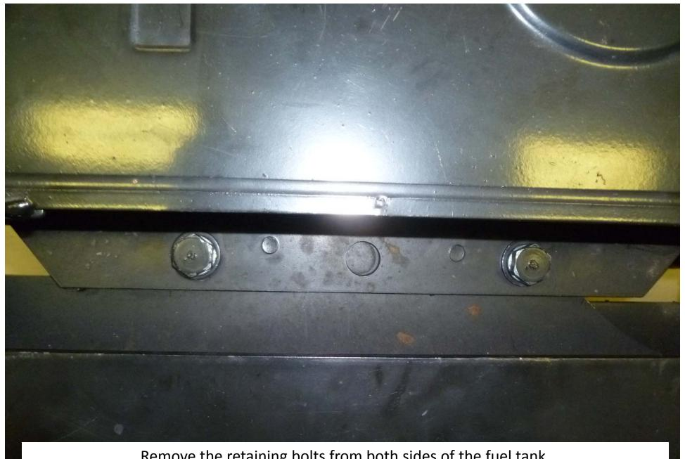
Remove the retaining bolts from both sides of the fuel tank.
