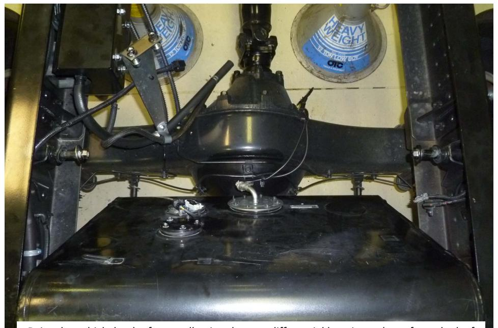
Raise the vehicle by the frame, allowing the rear differential housing to hang from the leaf springs. Support the vehicle with suitable jack stands under the frame.
