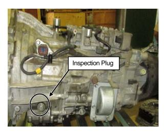
Circulate the ATF through the valve body and oil cooler
