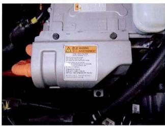
Pull out the yellow tab and pull up on the black tab and remove the EV motor power cable from the HPCU Assembly.
