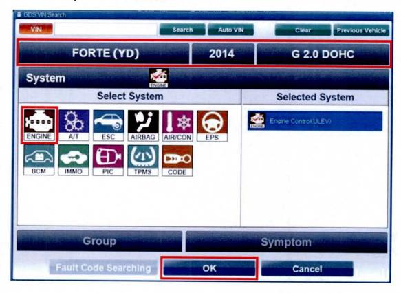
Select ECU Upgrade from the bottom right-hand corner. Next select Auto Mode, and then Engine. Perform the ECM upgrade in accordance with normal GDS ECM upgrade procedures.
