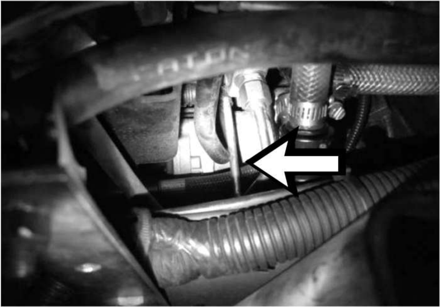
Illustration 1 Example of an AFI Fuel Supply Line rubbing
