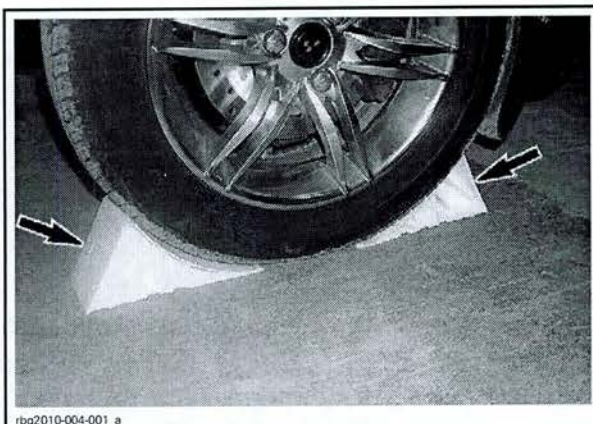
WHEEL CHOCK INSTALLATION, EACH FRONT WHEEL
