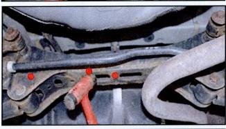
3. Use a wire brush or clean rag to remove debris from the front and rear crossmembers, front lower arms, rear upper and lower arms, and fuel tank.
