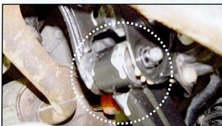
9. Spray the black undercoating on all exterior surfaces of the front and rear crossmembers, front lower arms, rear upper and lower arms and fuel tank. Refer to the photos on the right.
