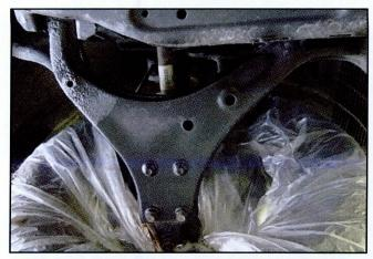
Rear crossmember, left and right rear suspension, left and right trailing arms, and brackets.
