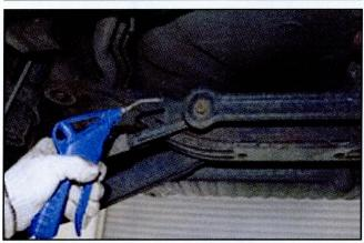
Top, bottom and sides of the fuel tank (M).
