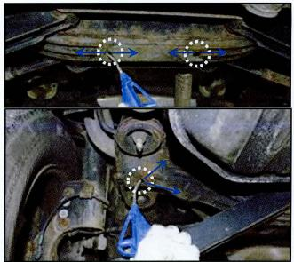
Exterior of left and right rear suspension, left and right trailing arms, and brackets.
