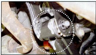
9. Spray the black undercoating on all exterior surfaces of the front and rear crossmembers, front lower arms, and rear suspension and trailing arms, brackets, and fuel tank. Refer to the photos on the right.
