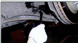
4. Remove the remaining debris in the components by inserting an air gun into the circled holes. Blow the air in multiple directions to remove as much debris as possible. Refer to the photos on the right.
