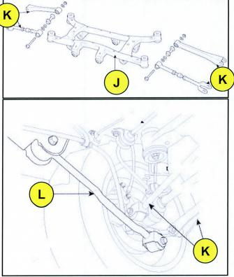
3. Use a wire brush or clean rag to remove debris from the front and rear crossmembers, front lower arms, rear suspension arms, rear trailing arms, brackets, and fuel tank.
