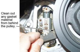
5. Turn the crankshaft counterclockwise until the cam chain auto-tensioner is compressed.
