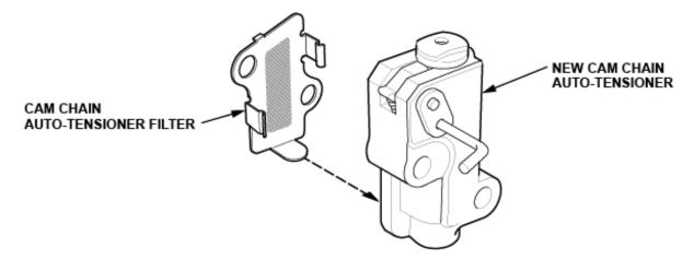
13. Install the new cam chain auto-tensioner with filter, and torque the bolts to 12 N·m (9 lb-ft).
