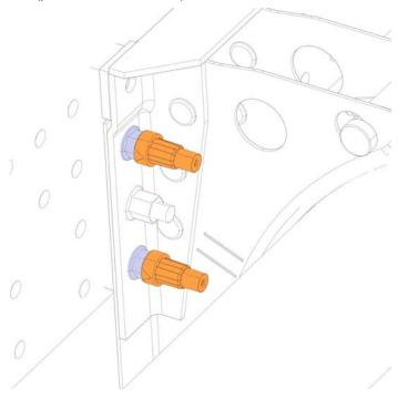
4 Install the filter on the mounting sleeves.
