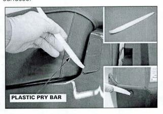
The plastic pry bar shown can also be used to lift the center pin of some common trim clips. Available in packs of 10 from the Honda Tool & Equipment program.
