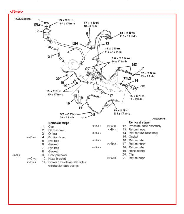
Please make the following additions and changes to the 2007–2013 Outlander Service Manual, Group 37 – Power Steering —> Power Steering Hoses —> Removal and Installation —> Removal Service Points -> >A<< Heat Protector/Pressure Hose Assembly/Return Tube Assembly/Return Tube Removal
