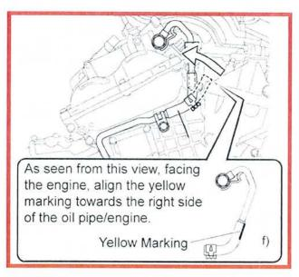
f) Install the oil hose's <u>vellow marking (upper) side</u> onto the upper oil pipe until it touches the spool. Align the <u>vellow marking</u> as illustrated.
