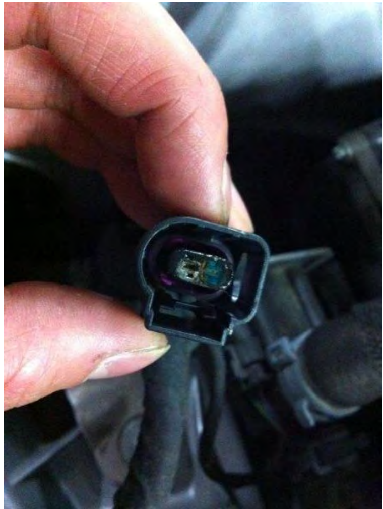
Figure 2. Corrosion formation on the connector pins.
