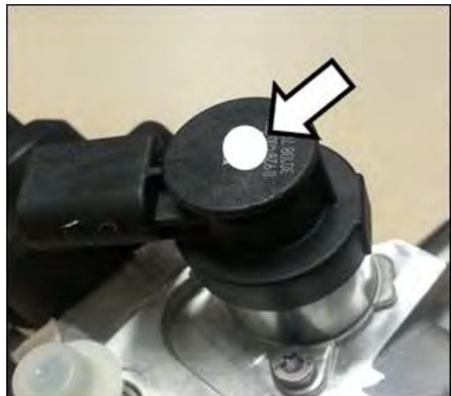
Figure 6. White dot on N290 fuel metering valve.
