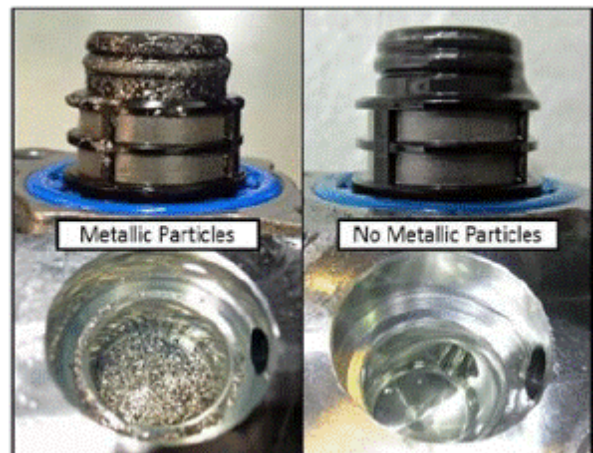
Figure 2. N290 fuel metering valve and valve bore shown with and without metallic particles.
