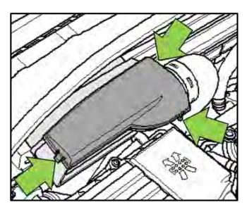
Reinstall the air duct cover and refasten the side clips <arrows>.
