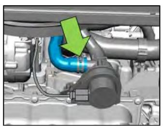
Reinstall the lower coolant hose onto the After-Run Coolant Pump V51 <arrow> and fasten the clamp.
