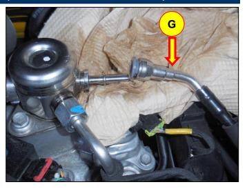
7. Disconnect the fuel feed tube quick-connector (G).
