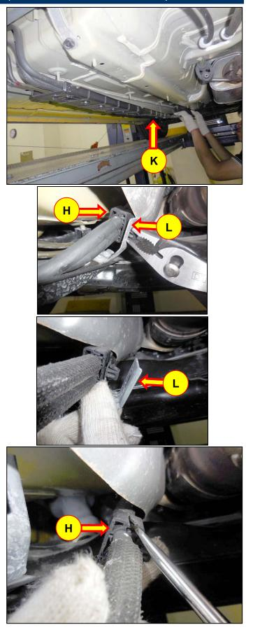
11. Release the holder (H) clip and separate the fuel feed tube from the holder.
