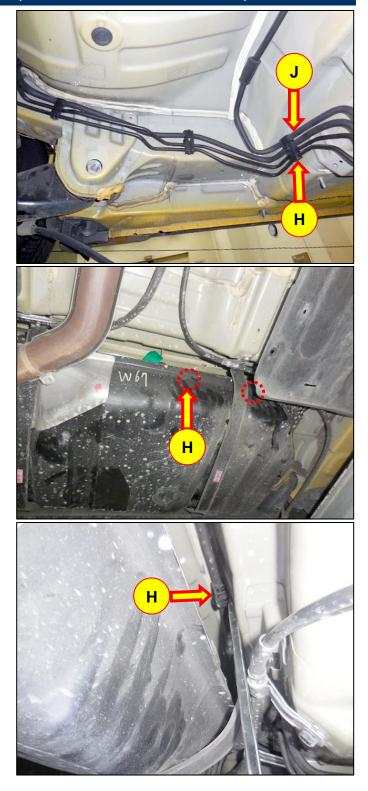
19. Separate the fuel feed tube (J) from the holder (H).
