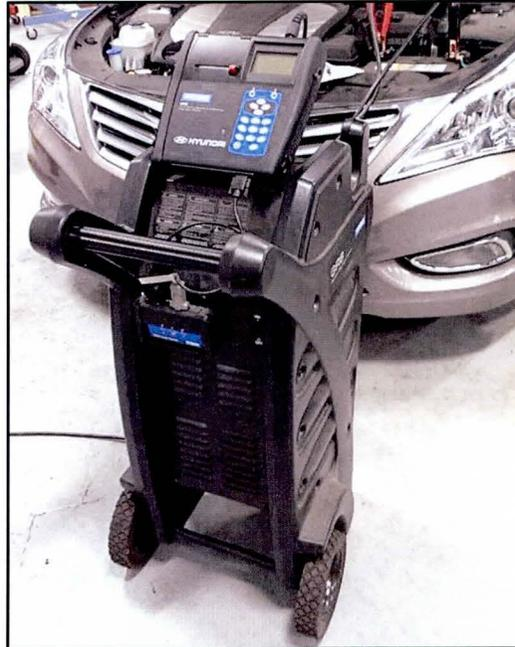
**GR8 Battery Tester Unit:** Performs battery testing and initial control of the diagnostic charger. Tester can be used independent of the charger unit after a battery charge is in process. The cable from the base may be disconnected and wireless communication exists to the Charger unit. The cable should be reconnected when docked on the charger.
