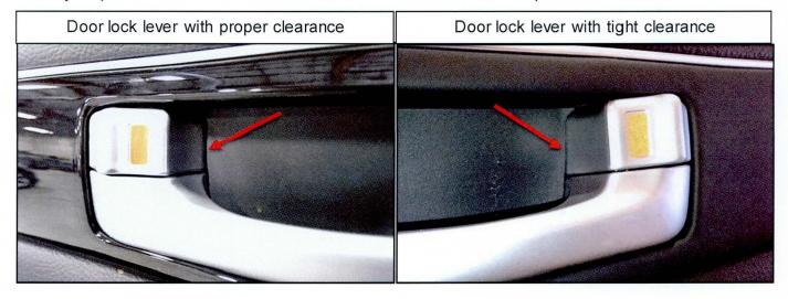
If the door lock lever has little or no clearance, or is jamming against the cap cover, proceed to the repair procedure described below.
