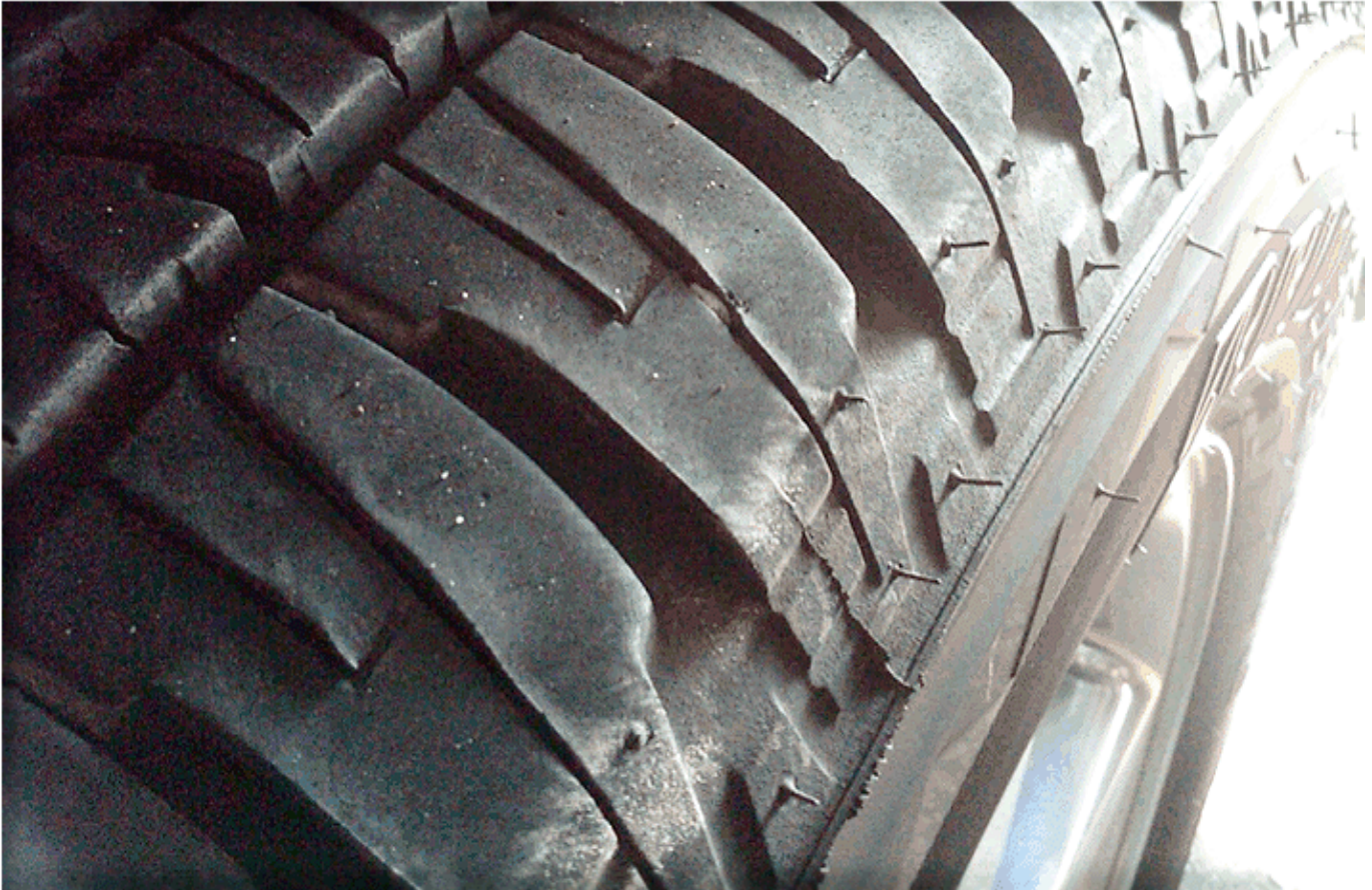
Figure 3: Tire Shoulder View Example 2 - "NORMAL" Tire "Feathering" Wear
