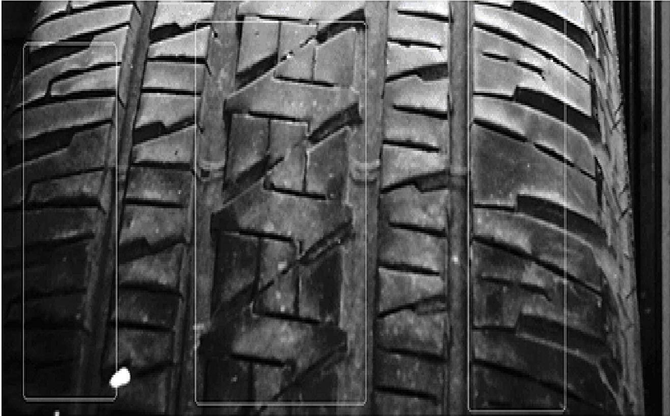
Figure 1: Full Tread View – “NORMAL” Tire “Feathering” Wear on the Shoulder/Adjacent/Center Ribs
