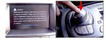
4.20 Enter the software update menu by simultaneously pressing the [B] DISC/AUX, [C] BACK, [D]NAVI/MENU buttons while pressing the [A] VOL KNOB.
