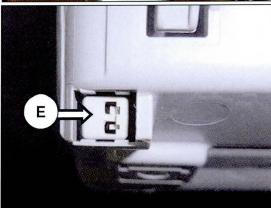
6. Push the back side of the holder latch (E) with a driver (F) to remove the holder latch from the overhead console.
