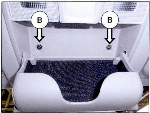
3. Pull down the overhead console (C) to separate it from the headliner.
