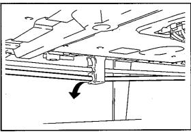
B. Using the SST, disconnect the left end of the luggage door hinge Torsion Bar LH from the luggage door hinge and the vehicle body.
