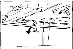
B. Using the SST, disconnect the right end of the luggage door hinge Torsion Bar RH from the luggage door hinge and the vehicle body.
