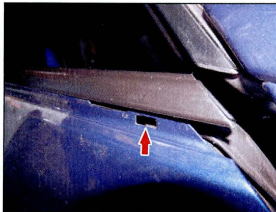
Figure 11. Hole for Clip in Outer Door Weatherstrip at Front of Door
