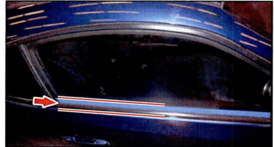
Figure 5. No Gap Between Tape and Outer Door Weatherstrip
