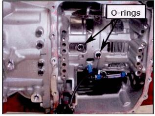
20. Align the manual shaft to the shift lever and install the valve body.
