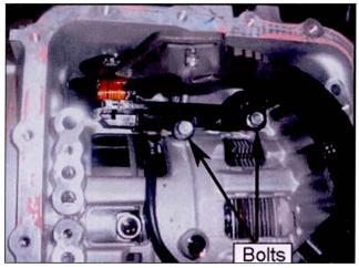
18. Remove two bolts that secure the input and output speed sensor and remove the sensor.
