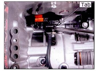
17. Remove two bolts that secure the valve body harness to the case.
