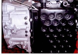
11. Use a small screwdriver to pry the connector from the oil temperature sensor (except for vehicles with integrated temperature sensor and harness).
